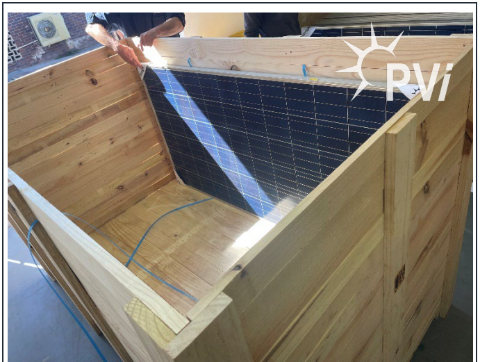
Modules placed in crate. Outside modules must be packed sunny-side facing in.
